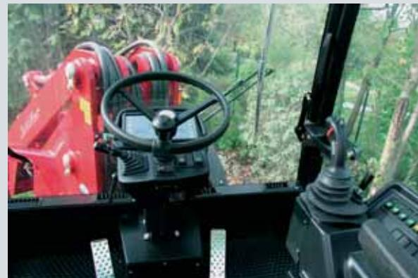
Hydraulically pre-controlled valves make work with a 9100 Z a pure pleasure. The absolutely delicate dosage of the work hydraulics by means of one hand joy-stick and exactly defined pressure points aren't only more comfortable but also safer. The spacious and comfortable cabin keeps the driver fit longer.
